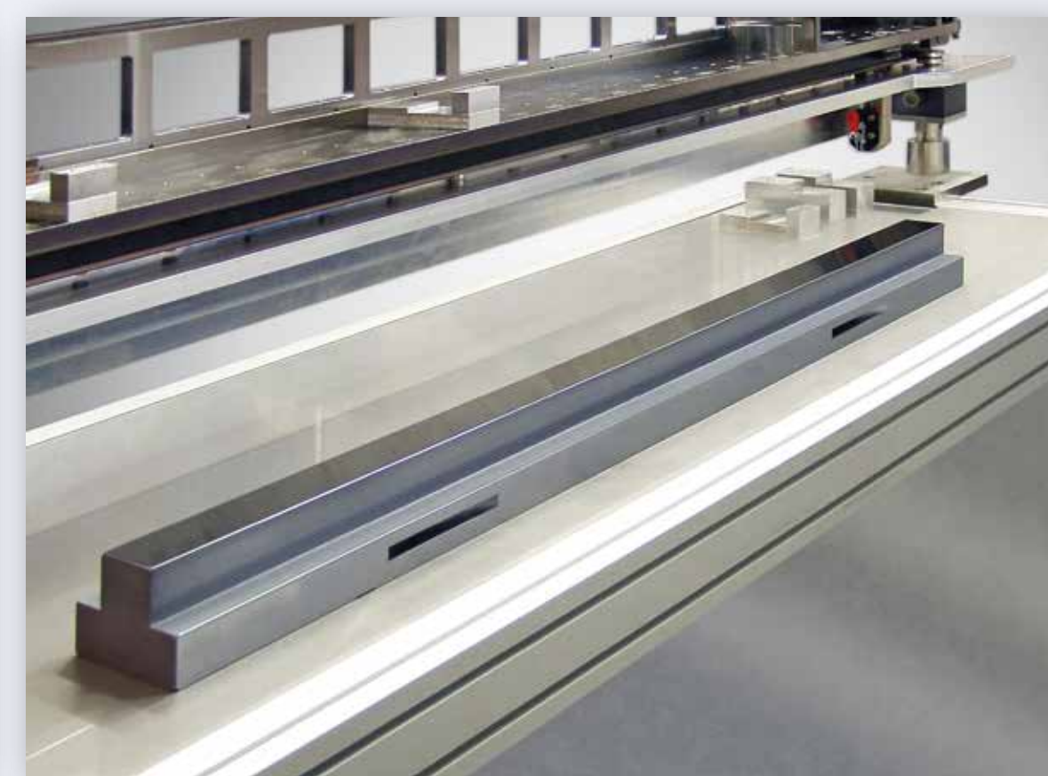
1000 mm Si mirror with special carbon coating.
