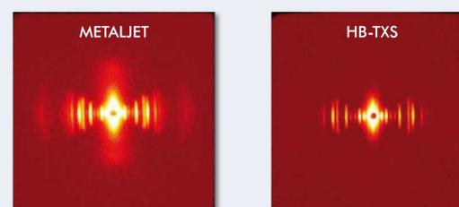
SAXS scattering plots of a very thin fiber from a rat tail tendon, measured with a Bruker AXS NANOSTAR equipped with the METALJET X-ray source (200 W at 70 kV) and the microfocus rotating anode TXS (2.5 W at 50 kV). Both use the same type of parallel Montel optics. The METALJET delivers 3x higher intensity.
