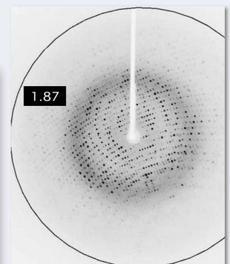
Data statistics and typical diffraction pattern of a protein complex, recorded with a D8 VENTURE 2<sup>nd</sup> Gen. and the METALJET X-ray source using a Ga rich alloy. The good data quality allowed for a structure solution by molecular replacement.
