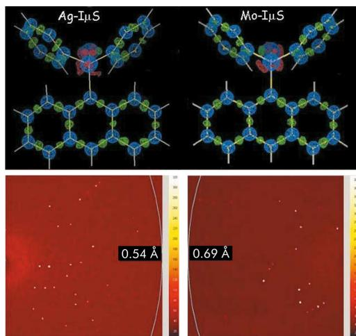
Figure 2: Comparison of the residual density and the resolution limit (at  $2\theta = 31^\circ$ ;  $\text{DX} = 51$  mm) for  $\text{C}_{26}\text{H}_{19}\text{PS}$ : Ag- $\mu\text{S}$  (200 s/°, left), Mo- $\mu\text{S}$  (77 s/°, right)
