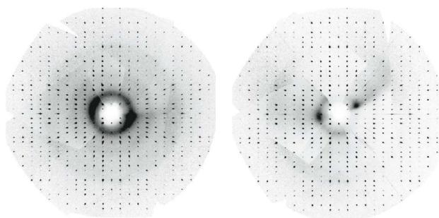
Figure 1: Calculated precession plots of the  $hk0$  layer for an organic sample: Mo-Sealed Tube (67 s/°, left), Mo- $\mu\text{S}$  (16 s/°, right)
