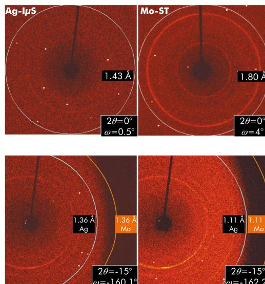
Figure 3: Diffraction patterns of a gabapentin heptahydrate single crystal in a DAC: top: comparison of Ag- $\mu\text{S}$  (20 s, left) against Mo sealed tube (20 s, right); below: diffraction patterns recorded with the Ag- $\mu\text{S}$  illustrating the gain in resolution with Ag-radiation.
