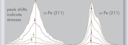
Scans in Steps of 100  $\mu\text{m}$  at the Transition between Ferrite (Axis) and Austenite (Turbine).
