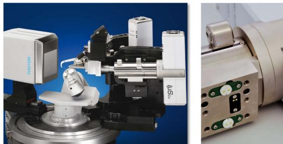
$\mu$ S integrated in a new Bruker D8 DISCOVER (left) and component recognition (right)
