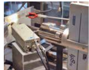
Combined XRF/XRD setup with Ag- \mu S, Univ. of Antwerp
