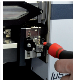
Quick-lock concept for easy alignment and serviceability
