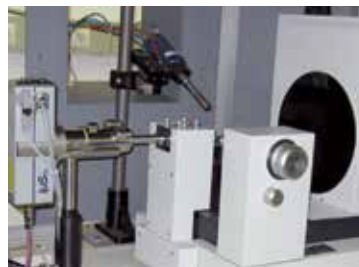
Before the upgrade: Standard mar345 with Rigaku RU 200 (Prof. P. Charlier, Uni- versity of Liège).
