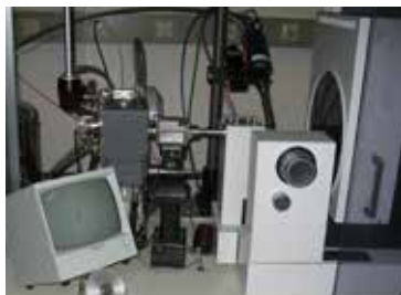
Before the upgrade: Standard mar345 with Rigaku RU 200 (Prof. P. Charlier, Uni- versity of Liège).
