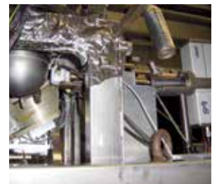
Surface and thin film XRD setup in Halle, Germany
