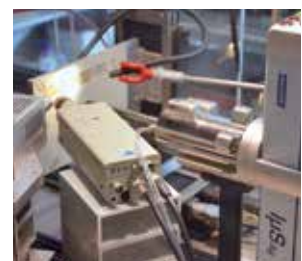
Combined XRF/XRD setup for painting analysis in Antwerp, Belgium
