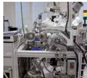
Adaptation to UHV deposition chamber for in-situ studies in Bratislava, Slovakia
