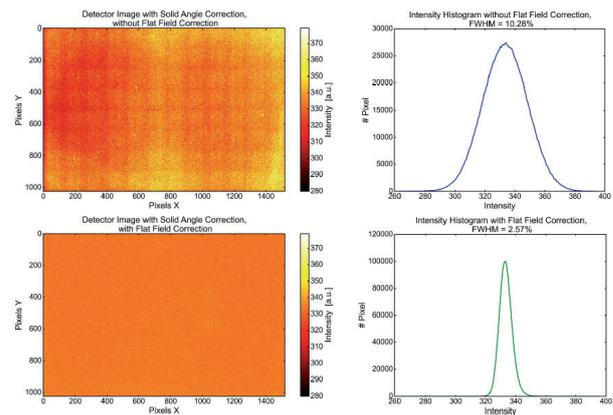
Comparison of two 1000 s images, one without flat field correction (top) and one with flat field correction applied (bottom), together with the corresponding intensity variation over the whole image. As can be seen from the histograms, the homogeneity in the intensity distribution is improved significantly by applying the flat field correction.
