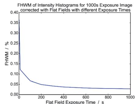
Improvement of the intensity homogeneity in dependence of the exposure time of the actual flat field image used for the correction. Reasonable statistics for the flat field correction are already obtained after about 10 min.
