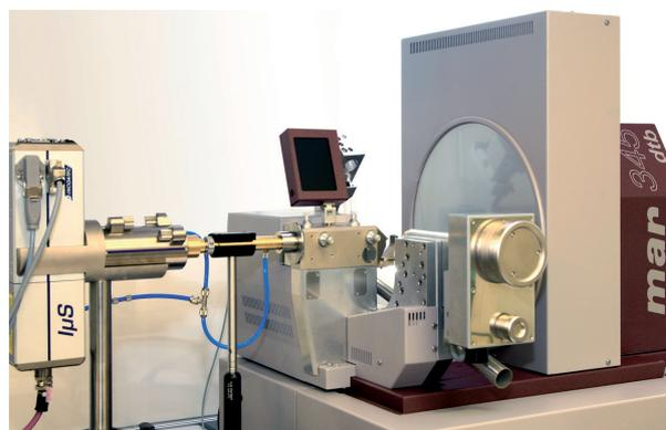
Figure 1: Incoatec Microfocus Source 1µS in combination with a mar research desktop beamline and an imaging plate detector mar345
